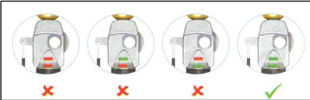
>If both indicators are red the Co2 gas cylinder must be replaced with a new one which must be of the same size. The automatic firing cartridge must also be replaced with
